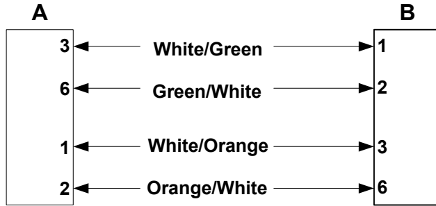
Figure 3-11. Pinouts for a Crossover Ethernet Cable
