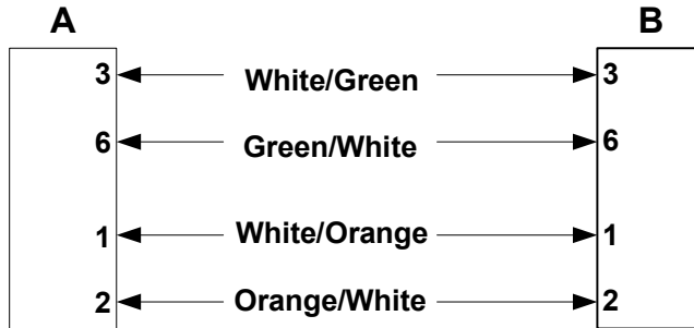
Figure 3-13. Pinouts for a straight-through Ethernet cable
