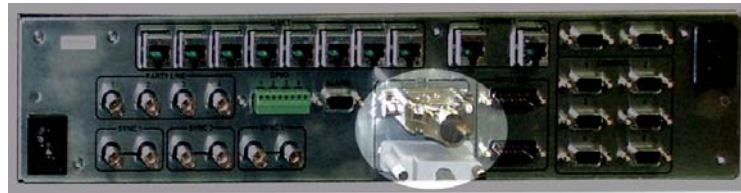
Figure 3-8. The MX-Bus Connectors (SC-4 rear)
